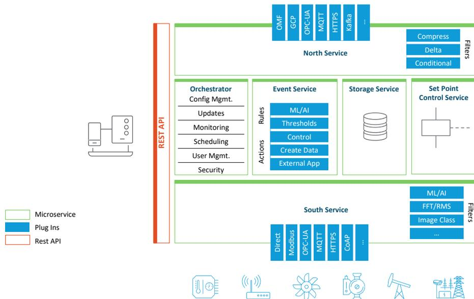
Readings can also be created in a filter pipeline or as a result of a notification. Knowing where in the lifecycle of a reading traversing through Fledge it may be processed and what off the shelf facilities exist for processing the data is recommended. These readings then pass through elements of the Fledge system before eventually being sent north to one or more external systems or being removed by a filter somewhere within a filter pipeline.
