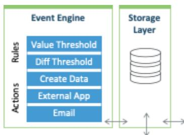
Fledge supports an optional microservice that is used to generate notifications or events. The notification service sits logically in the dataflow between the south ingress services and the storage service. It receives the data after it has been through ingress processing in the south services but before it has been processed for egress. As a result any processing done in south services is
