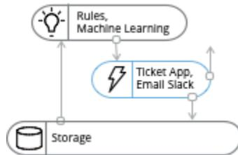
The notification service receives data that flows into the Fledge buffer and passes this to the various rules that have been configured for evaluation. If a rule is triggered then the delivery plugin associated with the notification is called to perform the action associated with that notification. Both notification rules and notification delivery mechanisms are implemented as plugins to the notification service and are thus extendable in the same way as other services within Fledge.
