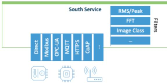
The filters may be arranged in a pipeline, such that the data that is read from the device is fed into the first filter in the pipeline, the data that comes out of that first filter is then fed into the second and so forth until the final filter in the pipeline. The output of the final filter is then sent to the storage service for buffering.
