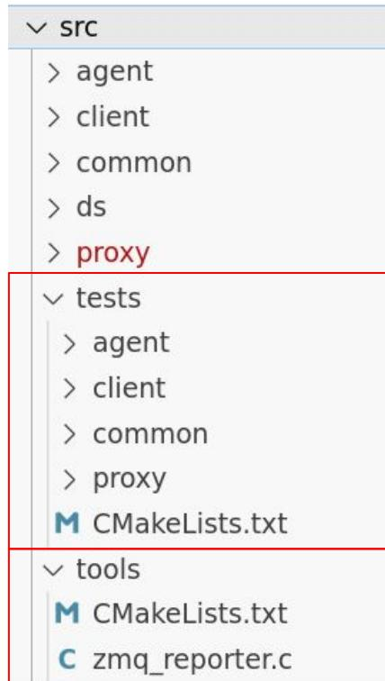
Unit Tests by components: agent, client, shared code (common), and proxy
