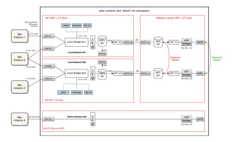
Special attention should be given to VPN networks. For the most part, these networks would be extended with VRFs just like the local network instances. However, for strongSwan (IKE daemon) to operate in multi-VRF mode, we have to switch to **Route-based VPN mode**. Using a special **XFRM device** (an enhanced alternative to VTI device), it is possible to bind an IPsec tunnel with a VRF domain as shown in the diagram below.
