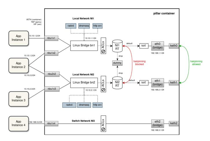
Note that the ACLs are mostly implemented on the network-instance side to provide drop and rate limiting, and also to mark packets for flowlog. There are a few iptables rules on the uplink (right) side to block some TCP/UDP ports from remote access etc.
