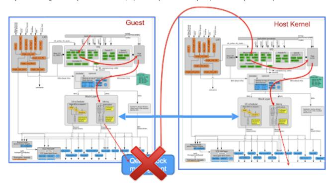
The diagram above shows a typical flow of the disk access of an application running in a virtual machine. The request would have to go through 3 software stacks
