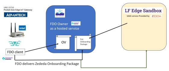
Zededa ZT Flow using Onboarding Package
